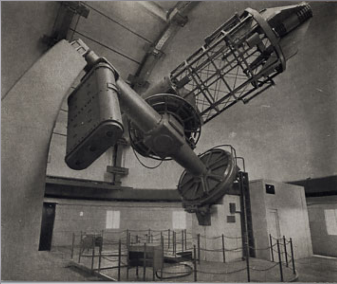
THE 82-INCH REFLECTING TELESCOPE OF THE W. J. McDONALD OBSERVATORY OF THE UNIVERSITY OF TEXAS. THE 82-INCH CONCAVE MIRROR, MADE OF PYREX GLASS, IS 11 AND THREE FOURTHS INCHES THICK AT THE EDGE AND WEIGHS ABOUT 5600 POUNDS.
